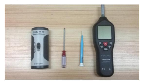
Step 1:Use the Metal screwdriver open the back cover of meter.
